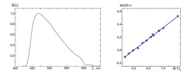
Figure 1.5: On left: Spectral response of the MASS device. On right: Color equation between MASS magnitude and star color index B-V.
