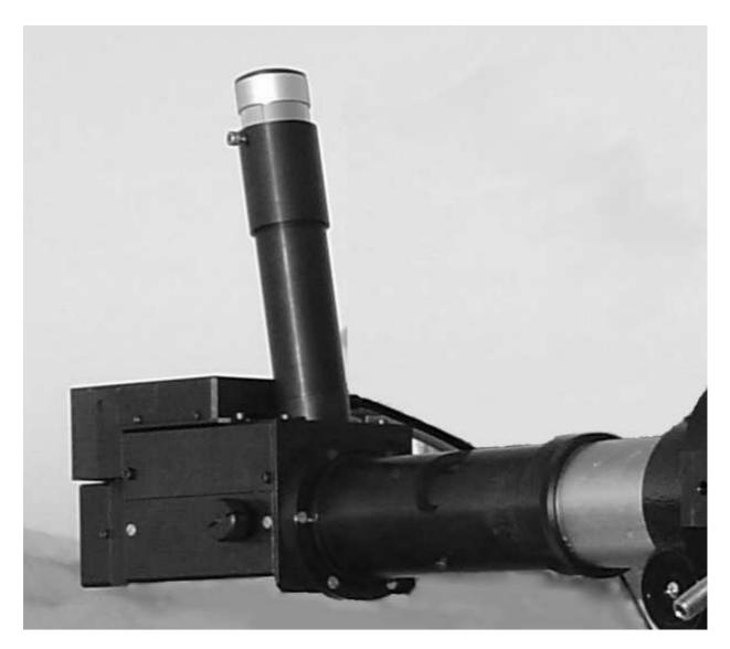
Figure 2.1: MASS device attached to refractor, which is installed atop of the La Silla DIMM.
