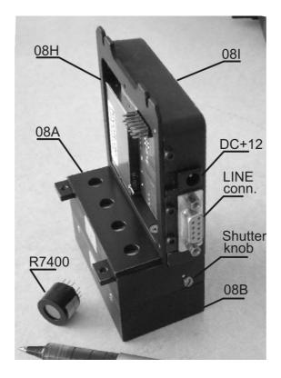
Figure 2.5: View of the detached electronics module. A photomultiplier PMT R7400 is shown separately. A pen on the photo is placed for comparison.
