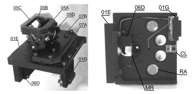
Figure 2.4: The top (left) and bottom (right) views of the optical bench. Star centering unit is removed.
