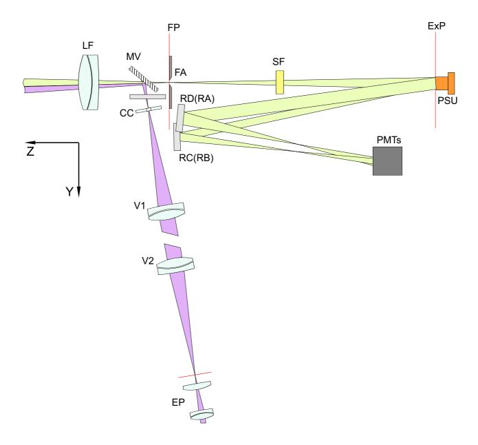
Figure 1.2: Optical layout of MASS device in ZY plane. LF — Fabry lens, FP — instrument focal plane, FA — field aperture, ExP — plane of exit pupil, PSU — pupil segmentation unit, RA, RB, RC, RD — re-imaging mirrors, SF — spectral filter, PMTs — MASS detectors, MV — viewer removable mirror, CC – glass plate with central hole, V1, V2 — transmoving objective, EP — eye-piece.
