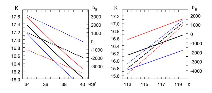
Figure 3.2: System magnification K (solid line) and entrance pupil plane position  $b_E$  (dashed line) dependence on the Fabry lens focusing (left) and transfocator lens position c (right). -da' is a distance between the device focal plane and LF. c is a distance between the device focal plane and LF. c is a distance between the device focal plane and TF. Black line — for nominal focal lengths (60 mm and -18 mm), blue — at 1.5% less, red — at 1.5% greater.
