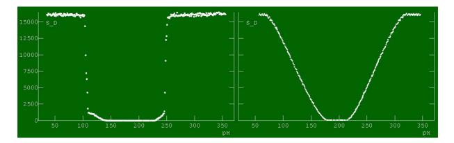
Figure 1.6: Image scans produced by centering mechanism. On left — scan of a point-like image, on right — scan of uniformly illuminated aperture.
