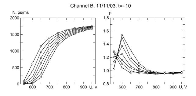
Figure 4.1: Light counting functions. Left: Flux dependence on the high voltage for 7 threshold levels (0.3, 0.4, 0.5, 0.6, 0.7, 0.8 and 0.9 mV), lowest curve corresponds to the 0.9 mV level. Right: Non-Poisson parameter as a function of Voltage for 7 threshold levels, here lowest curve corresponds to the 0.3 mV threshold.
