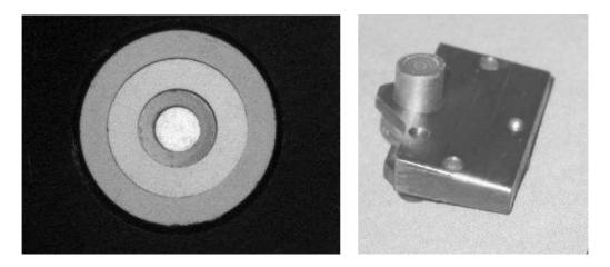
Figure 1.4: On the left: Top view of one of the MASS segmentator, illuminated by scattered light. On the right: Segmentator mounted in its holder.
