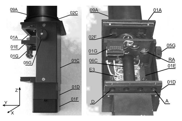
Figure 2.3: View of the device without cover. Used coordinate system is shown, too.
