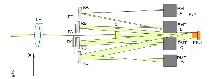
Figure 1.3: Optical layout of the MASS device in ZX plane (corresponds to the bottom view in Fig 1.2). Viewer is not shown. LF — Fabry lens, FP — instrument focal plane, FA — field aperture, TK — triangle knife of centering unit, ExP — plane of exit pupil, PSU — pupil segmentation unit, RA, RB, RC, RD — re-imaging mirrors of the A-, B-, C-, and D-channels, SF — spectral filter, PMT — four detectors.
