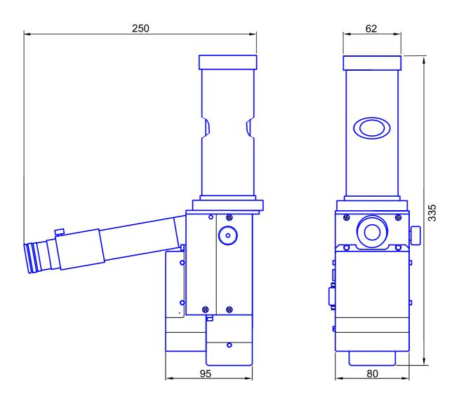
Figure 2.2: Main dimensions of the MASS device with optical interface.
