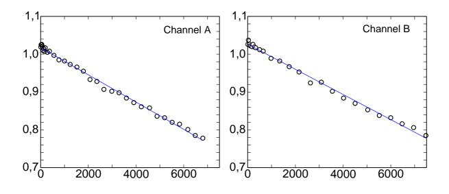
Figure 4.2: Dependence of non-Poisson parameter p on flux F for A and B channels. Line is linearly fitting the measured points.
