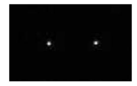
Figure 3.2: On left: The CCD frame of the illuminated field aperture. On right: Right aligned artifical star images with the horizontal separation of 41 pixels.
