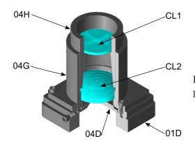
Figure 3.3: Wide field eye-piece for exit pupil alignments.
