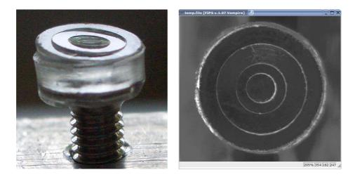
Figure 1.6: On the left: Side view of the one of the MASS segmentator mounted on its holder. On the right: Top view of the finished segmentator. The PSU is illuminated by scattered light.
