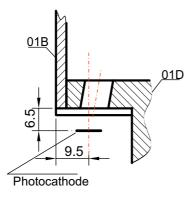
Figure 3.1: Photocathodes position with respect to the reference plate of the bottom tie.
