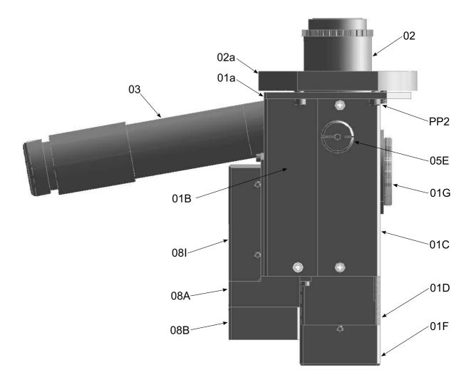
Figure 2.1: Side view of the MASS/DIMM device without CCD camera. See designations in text.
