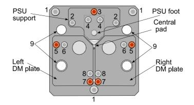
Figure 2.7: The optical plate with PSU in its holder and two DIMM mirrors alignment plates. 1 — screws M2.5 fixed plate to device, 2 — pull alignment screws M2 of the PSU support, 3 — push screw M2 for PSU tilt alignment, 4 — PSU lock screws, 5, 6 — push and pull screws M2 for alignment of the DIMM mirrors tilt in X direction, 7, 8 — push and pull screws M2 for alignment of the DIMM mirrors tilt in Y direction, 9 — windows for mask fixing screws.
