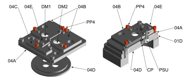
Figure 2.5: The view of the optical plate with PSU holder and two DIMM mirrors alignment plane.
