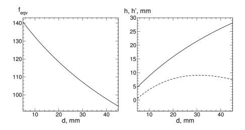
Figure 1.2: Dependence of the equivalent focal length of a complex Fabry lens (left) and position of principal points (solid — direct path, dashed — reverse) on the lens separation d
