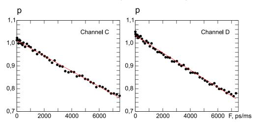
Figure 4.3: Dependence of non-Poisson parameter p on flux F for C and D channels. Line is linearly fitting the measured points.
