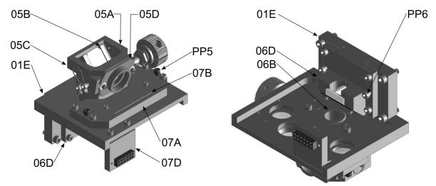
Figure 2.3: The top (left) and bottom (right) views of the optical bench.
