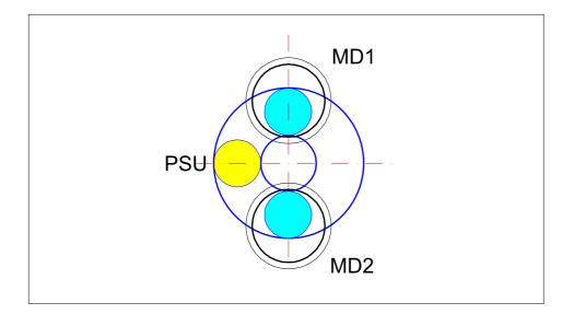
Figure 1.3: Geometry of exit pupil for telescope C11. MASS PSU is shown by yellow. DIMM masks are shown by cyan. Black — the placement of DIMM re-imaging mirrors.
