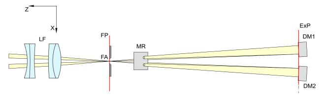
Figure 1.8: Optical layout of DIMM sub-device in ZX plane (corresponds to the top view in Fig 1.4). The MASS sub-device and viewer are not shown. Common part: LF — Fabry lens, FP — instrument focal plane, FA — field aperture, ExP — plane of exit pupil and mask. DIMM: DM1 and DM2 — DIMM re-imaging mirrors, MR — folding mirror.
