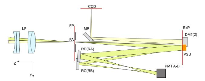
Figure 1.4: Optical layout of MASS/DIMM device in ZY plane. Common parts: LF — Fabry lens, FP — instrument focal plane, FA — field aperture, ExP — plane of exit pupil. MASS sub-device: PSU — pupil segmentation unit, RA, RB, RC, RD — re-imaging mirrors, PMTs — MASS detectors. DIMM sub-device: DMs — two DIMM re-imaging mirrors, MR — folding mirror, CCD — plane of CCD detector. Viewer is not shown.
