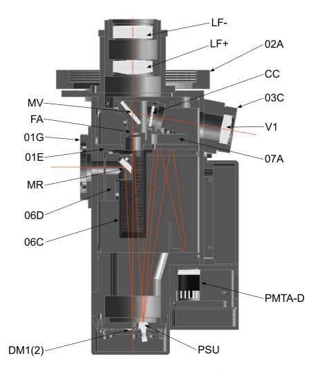
Figure 2.2: Cross-section view of the MASS/DIMM device.
