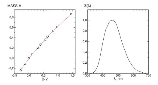
Figure 1.7: On left: Color equation between MASS magnitude and star color index B-V. On right: Spectral response of the ELT MASS device.
