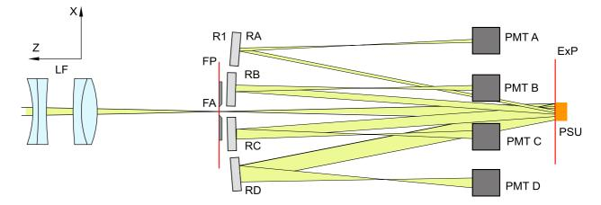
Figure 1.5: Optical layout of the MASS sub-device in ZX plane (corresponds to the bottom view in Fig 1.4). DIMM sub-device and viewer are not shown. Common part: LF — Fabry lens, FP — instrument focal plane, FA — field aperture, ExP — plane of exit pupil. MASS: PSU — pupil segmentation unit, RA, RB, RC, RD — re-imaging mirrors of the A-, B-, C-, and D-channels, PMT — four detectors.
