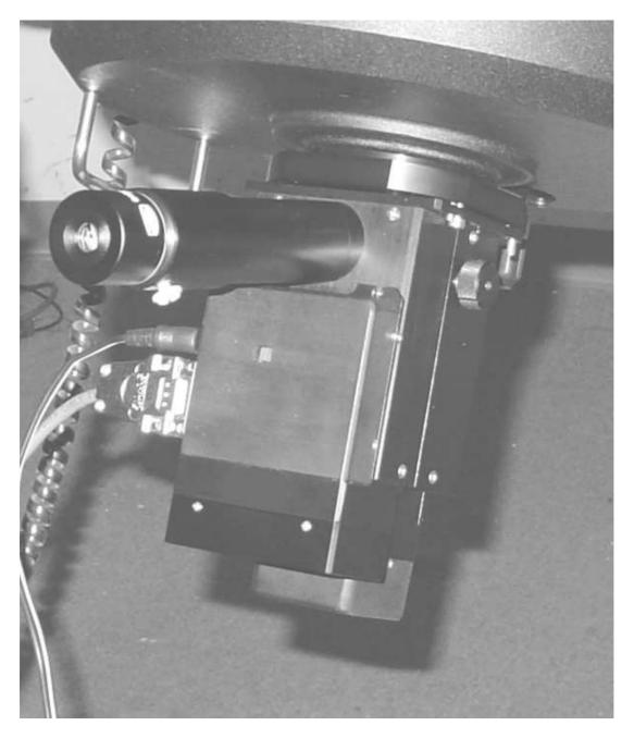
Figure 1.1: ELT MASS/DIMM device at the telescope C11. View from the side of the viewer and electronics box.
