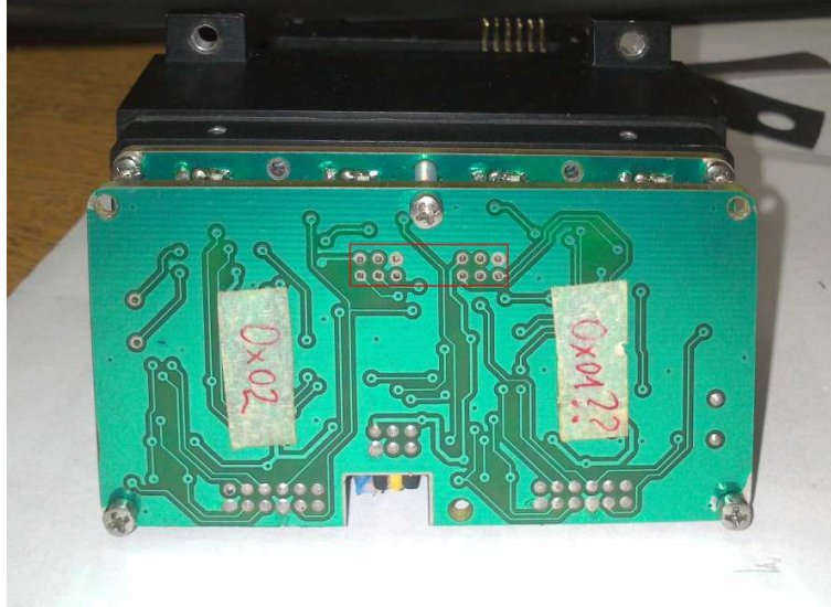
Figure 3: Counters circuit board with the 2-mm pitch ISP sockets (in the red box). The sockets of bic2 are on the left, the sockets of bic1 on the right.
