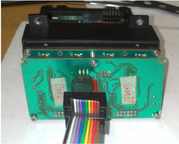
Figure 4: Connection of the programming adaptor to then sockets of bic2.
