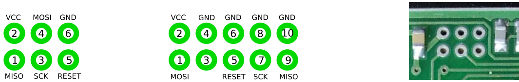
Figure 1: Pin layout of ISP6 and ISP10 connectors, looking top down to the PCB. Image on the right shows part of the MASS power module with ISP sockets, oriented in the same way as the ISP6 connector on the left.
